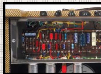
■ Both amps are entirely hand-wired, with the components neatly laid out on tag board
