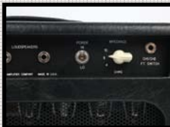
■ The half-power mode turns a pair of the output valves off giving around 18 watts of output
